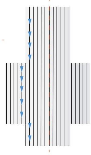
Fiber flow is cut during machining operations
